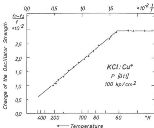
Fig. 2. Stress effect of the oscillator strength of the band at 4.7 eV in  $\text{KCl}:\text{Cu}^+$  versus temperature.
