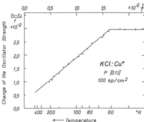
Fig. 2. Stress effect of the oscillator strength of the band at 4.7 eV in KCl:Cu<sup>+</sup> versus temperature.
